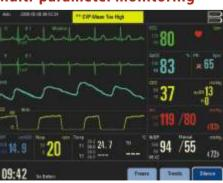
Diagnostic-quality measurements and monitoring including ECG, SpO<sub>2</sub>, NIBP, TEMP, RESP, IBP and EtCO<sub>2</sub>
