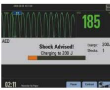
In AED mode, the defibrillator/monitor automatically analyzes the rhythm and determines whether a shock is advised. Voice and text prompts guide the user through the process. Voice recording is also available.
